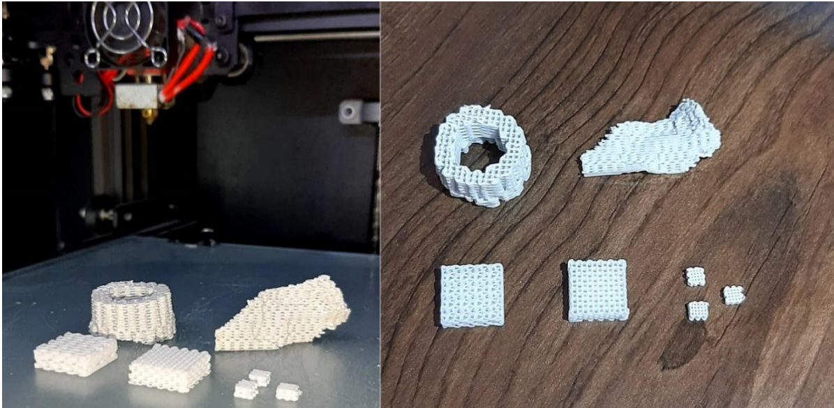
Figure 2. Left: Scaffolds on 3d printing bed at the end of the printing process, Right: Different scaffolds with diverse shape and pores. (Design by Authors - 2024)
